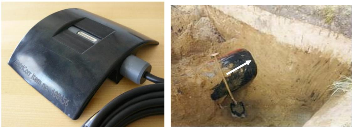
*Figure 2: Left: Rod type ER probe embedded in sleeve for the purpose of providing a better integration with a pipe surface. Right: Illustration relating to the installation during excavation procedures. In order to ensure installation in original backfill (or same soil as the pipeline) make the excavation in such manner that an original wall of soil is left behind in which the coupon is installed (white arrow indication)*
