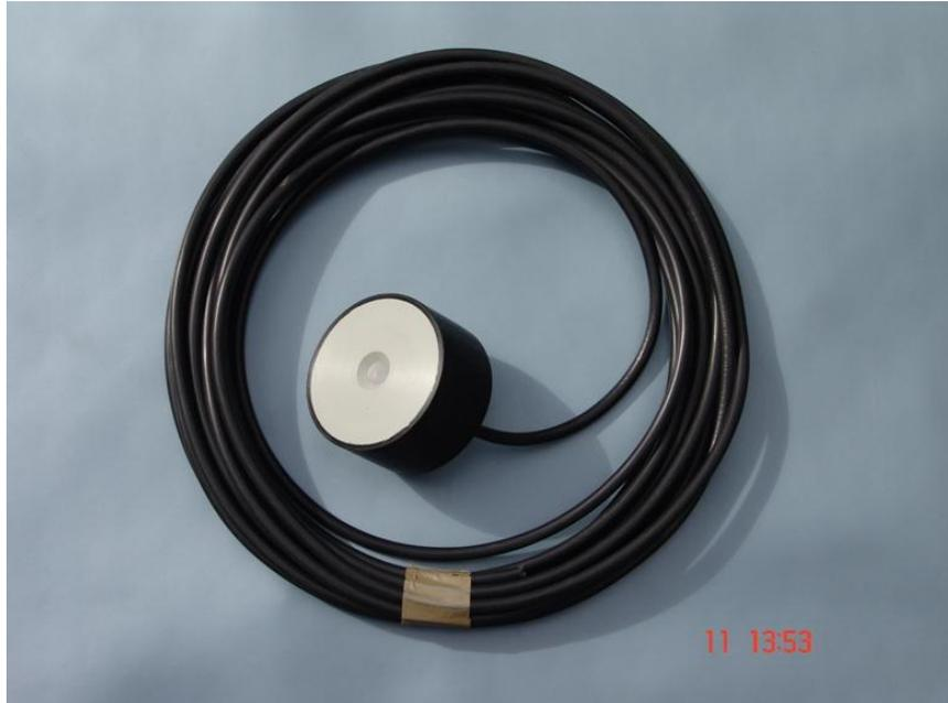
*Figure A1.3. Conductive perforation coupon.*
