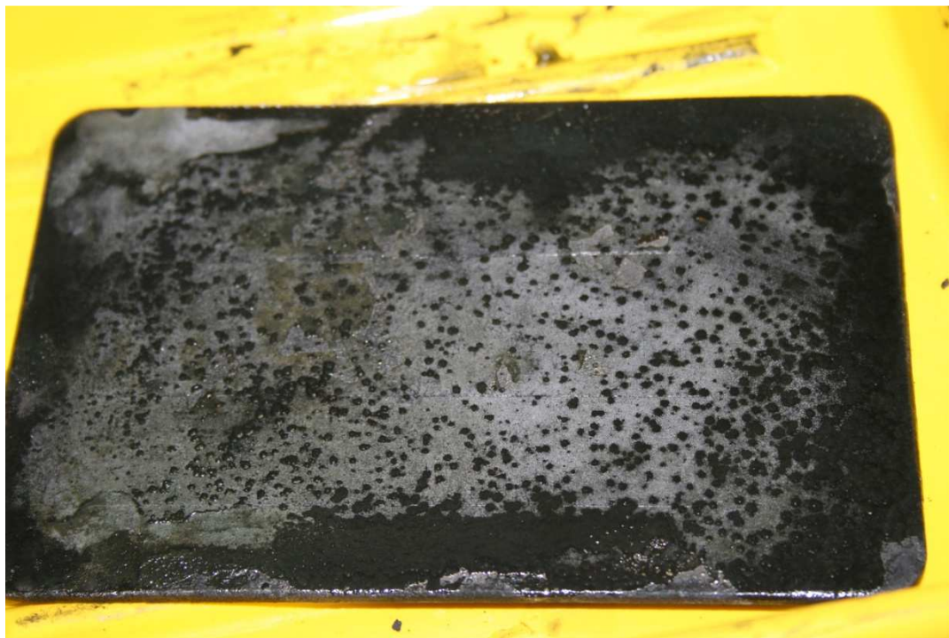
Figure 2: Ferrous sulfide and carbonate precipitate on an iron plate corroded by sulfate-reducing bacteria.
