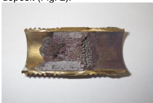
Fig. 2a: Fitting with voluminous deposit
